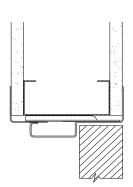
Wall Construction Metal Studs & Drywall Recommended Fasteners: 1-1/4" (min.) Type "S" Bugle Head Self-Tapping Screws
