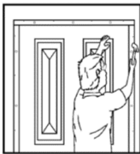
6 Fasten frame starting at top of hinge jamb
