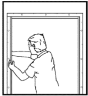
4. Place strike jamb over wall
