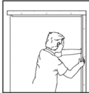
3. Place hinge jamb over wall
