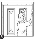
Using door as a template adjust frame to door so that clearances between door and the frame are equal and between 1/16" - 1/8". If a door is not available square and plumb the frame using a carpenter's square and level Fasten frame starting at top of the hinge jamb with recommended fasteners
