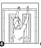
Remove nails or screws used to hold the header. Pull down on header so that the jambs rest on finished floor. If the finished floor is not installed, place a shim of the same thickness as finished floor, under each jamb. Insert one screw or nail at top of hinge iamb. Install door and close in opening.
