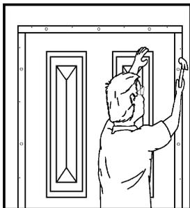
5 Fasten frame starting at top of hinge jamb
